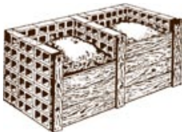
Concrete block bin
